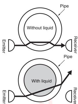
1. If there is no liquid in the pipe, the emitted beam will reach the receiver after it is refracted by the pipe. (Light incident.)
