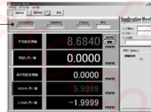
Application Monitor for Flatness Measurement
