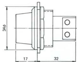
NEON PILOT LAMP 25mm $\phi$  Mounting Hole
